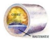
Wastewater collection lines are designed to handle three things; used water, human waste and toilet paper. It is very important to keep all foreign materials, such as grease and other household items, non-flushable products and debris from entering the sewer system.
